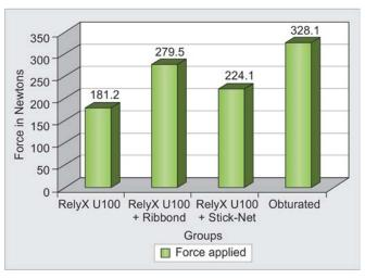
Graph 1: Mean vertical fracture strength of various fibers tested
