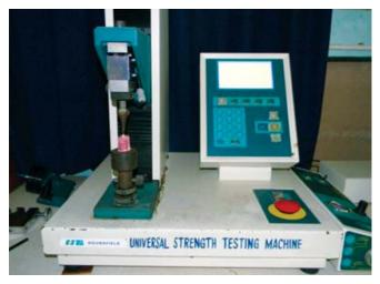
Fig. 2: Universal testing machine with acrylic resin block containing root segment
