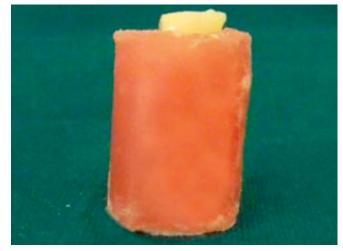
Fig. 1: Acrylic resin block containing root segment exposing 2 mm of coronal opening of the root for seating of loading device of universal testing machine for load to fracture test
