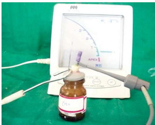
Fig. 1: Experimental model assembly for determination of electronic working length
