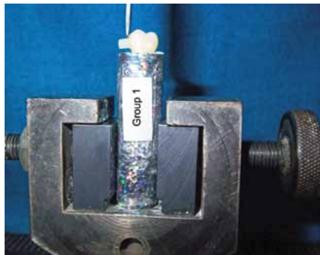
Fig. 6: Chisel at the crosshead speed of 0.5 mm/min of Lloyds LR100K universal testing machine
