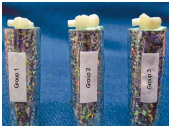
Fig. 3: Sealants of each group were filled into the plastic mold and cured
