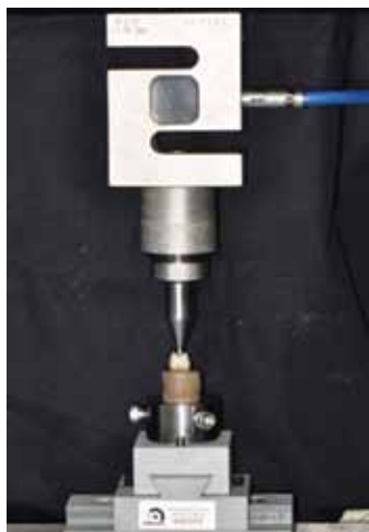
Fig. 2: Applying a static load to the sample with a universal testing machine
