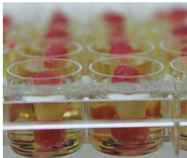
Fig. 1: Cell culture plates filled with BHI broth and specimens fixed with sticky wax
