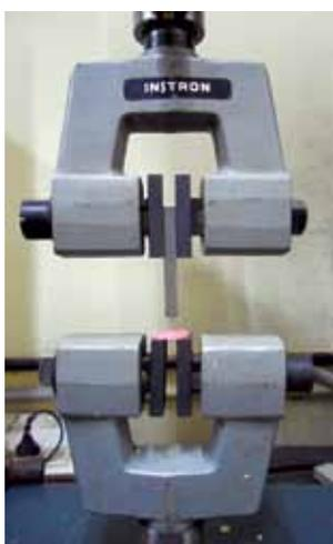
**Fig. 1:** Measurement of pushout bond strength using Instron Universal Testing Machine
