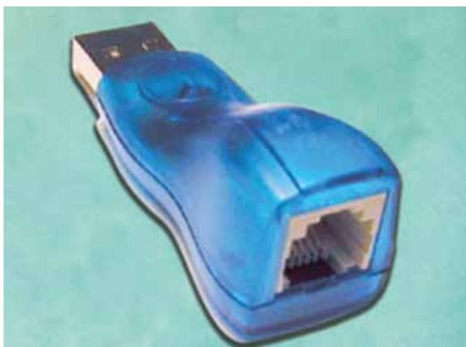
Fig. 7: The DS9490R USB adapter that attaches to the computer
