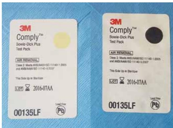
**Fig. 2A:** Bowie Dick type test pack that is used to test air removal in autoclaves that have a vacuum cycle
