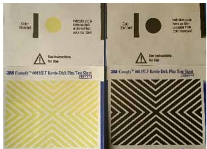
**Fig. 2B:** Bowie Dick test pack showing the indicators inside of the challenge pack that show uniform color change (from yellow transverse stripes changing to a black)
