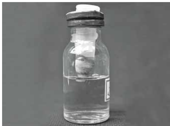
Fig. 1: Specimen showing apical portion of the teeth immersed in the culture medium, and the upper part mounted on the Eppendorf tube sealed with cyanocrylate and nail varnish, the tube-tooth unit is mounted inside the rubber cover and placed inside the glass flask.
