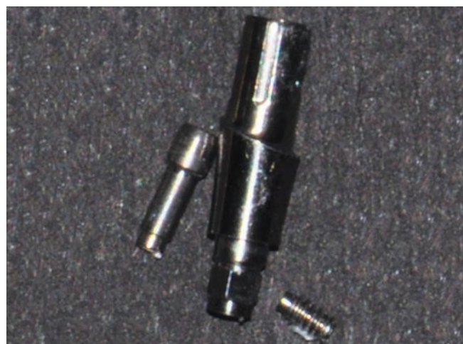
Fig. 2: Screw fracture in 3.4 mm titanium abutment
