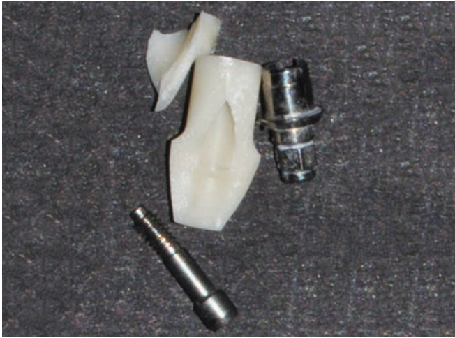
Fig. 3: Screw distortion and body fracture in 3.4 mm zirconia metal abutment
