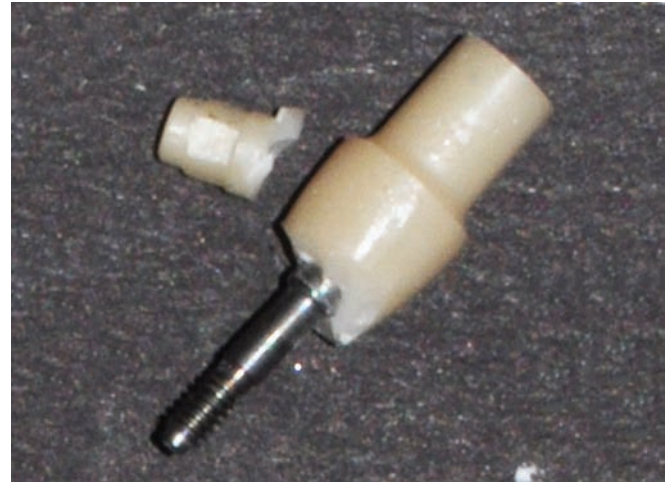
Fig. 4: Connection area fracture in 3.8 mm copy-milled abutment
