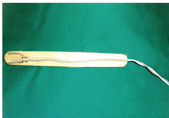
Fig. 3: Disposable probe made up of four 1-mm-diameter silver electrodes (2 mm distance between electrode centers) mounted in square configuration on a wooden spatula
