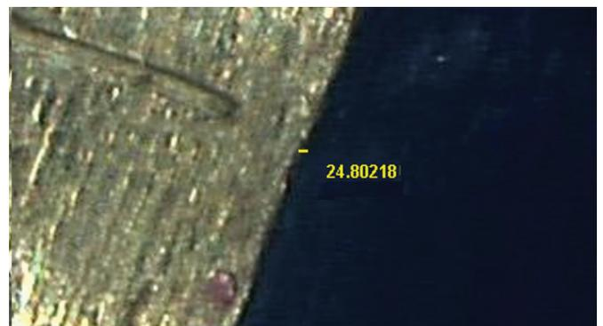
Fig. 3: The marginal discrepancy between the metal die and the wax pattern was measured on an optical stereomicroscope
