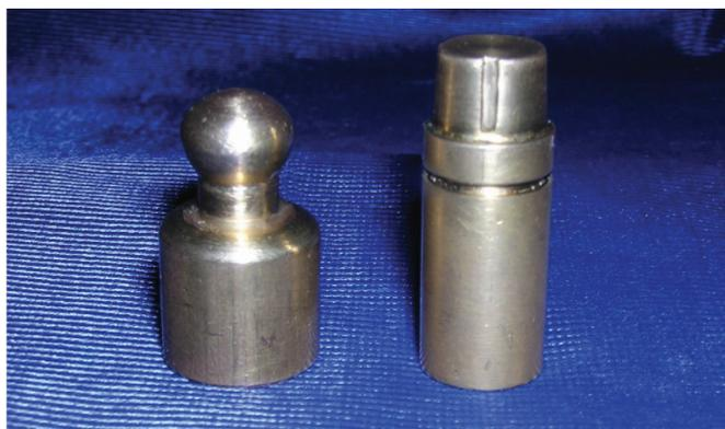
Fig. 1: Master model with counter die
