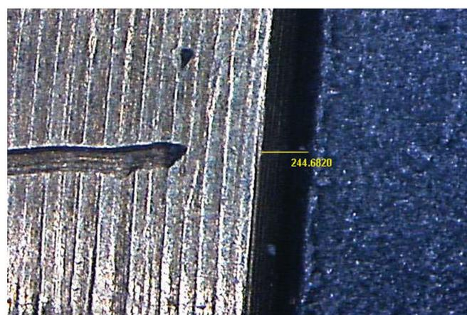
**Fig. 5:** The marginal discrepancy between the metal die and the casting was measured on an optical stereomicroscope
