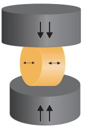
Fig. 2: Schematic illustration showing the mounting of sample to test DTS
