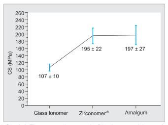
**Graph 1:** The compressive strength of the three materials tested
