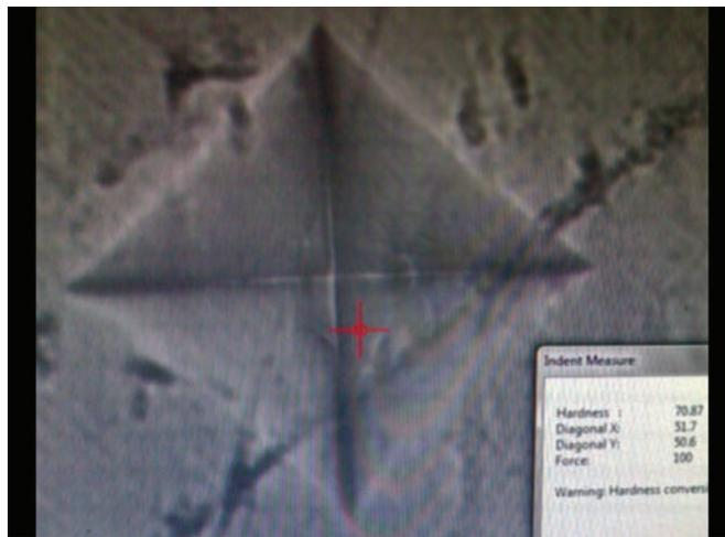
**Fig. 2:** Indentation of Vicker's Hardness needle
