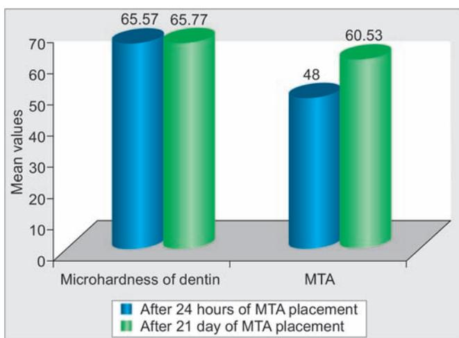
**Graph 1:** Comparison of mean baseline values of microhardness of dentin and MTA by Vicker's microhardness test at 100 gm weight for 5 seconds before exposure to acids after 24 hours of MTA placement and after 21 days of MTA placement
