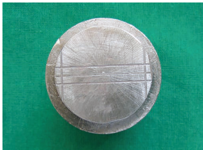
Fig. 1: ADA specification no. 18 master die
