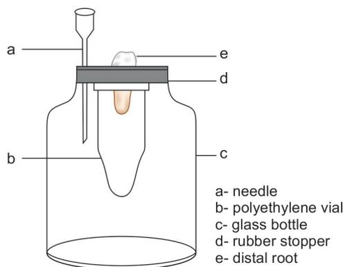
**Fig. 1:** Schematic representation of the apparatus designed by Myers and Montgomery, which was used for this study
