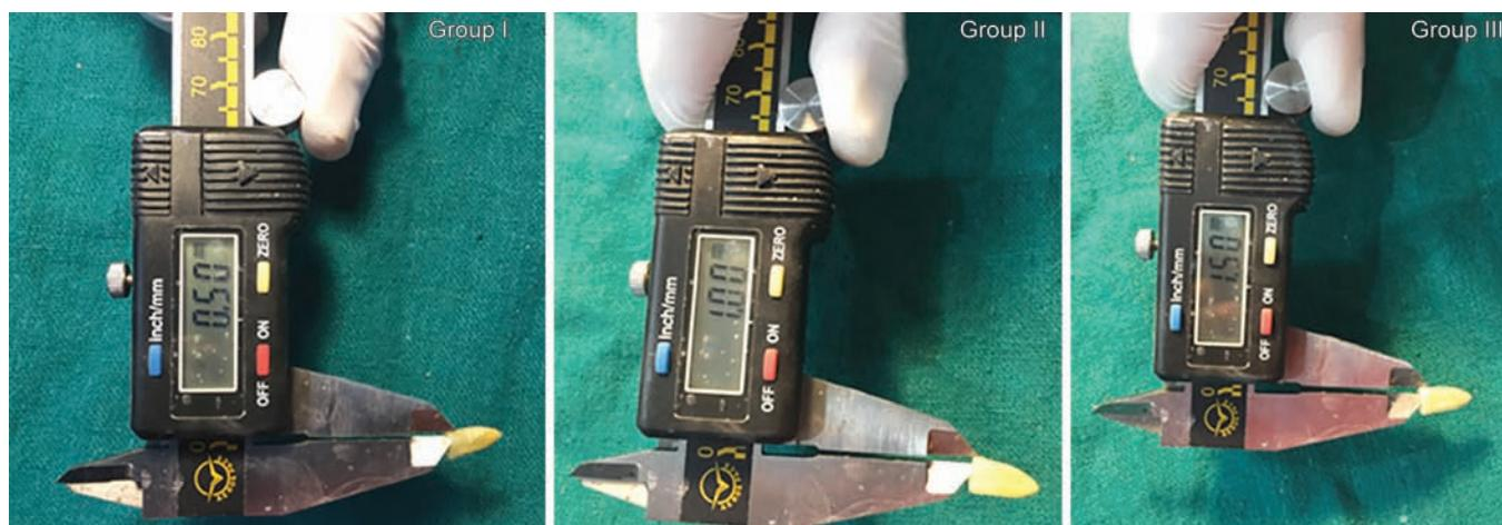
**Fig. 1:** Estimation of thickness of dentin in groups I, II, and III after post space preparation using digital Vernier caliper
