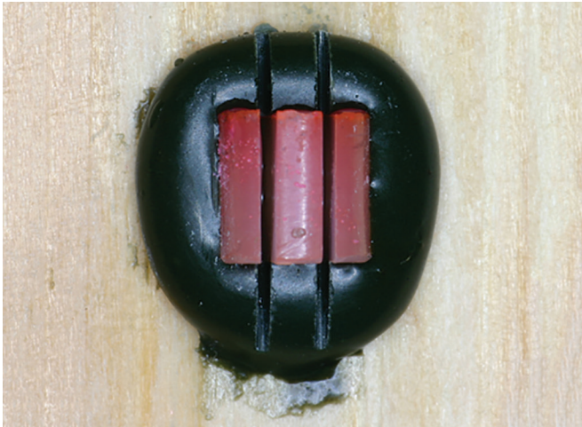
Fig. 3: A 1.5 mm slice of the composite polymerized and stained with the dye
