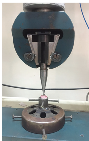
Fig. 4: Application of the load cell to the veneer until fracture in a universal testing machine
