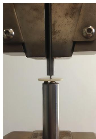
Fig. 2: Biaxial flexural strength testing using universal testing machine
