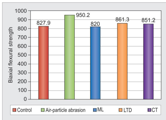
**Graph 1:** Comparison of biaxial flexural strength of Cercon® specimens after different surface treatments
