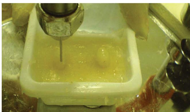
**Fig. 3:** Mounting in acrylic resin
