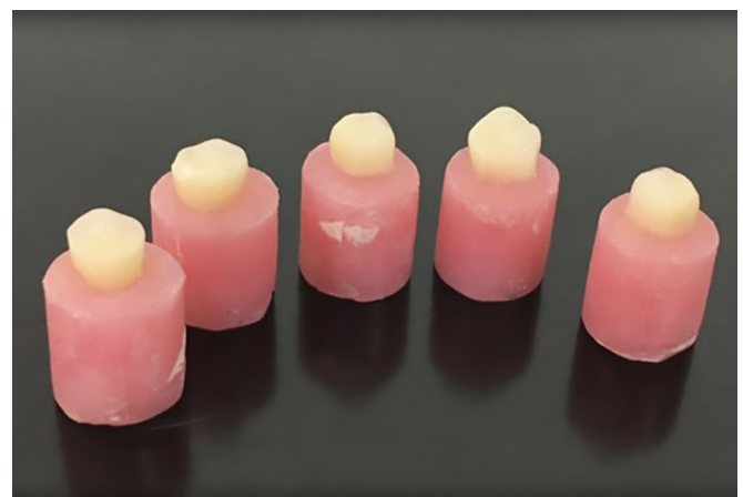
Fig. 1: Acrylic cylindrical denture base specimens with acrylic premolar teeth after surface conditioning treatment
