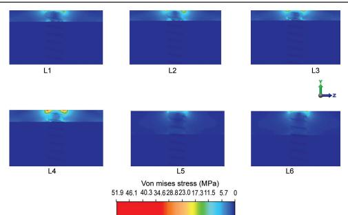
Fig. 3: von Mises stress field amplified in the cortical bone region
