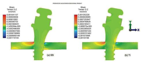
Fig. 5: Strain tensor z-z in the cortical bone region
