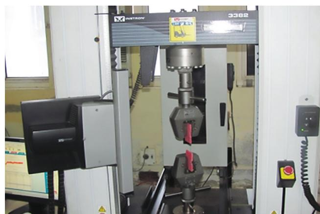
Fig. 3: Instron universal testing machine
