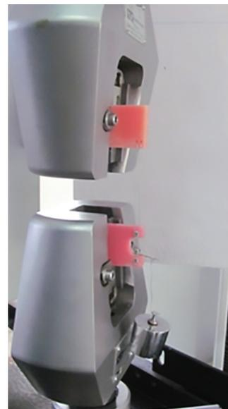
Fig. 2: Force application parallel to the bracket
